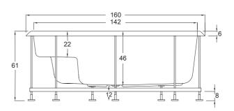
If the bath is recessed the masonry cannot reenter more than the masonry must fall back to the outer edge of 2 cm. An inspection panel and air intake must be installed.
