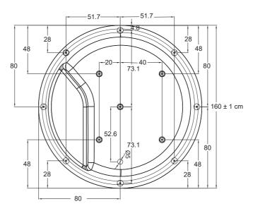
The overall dimensions are given in centimetres. Actual dimensions can vary by  $\pm$  1 cm.
